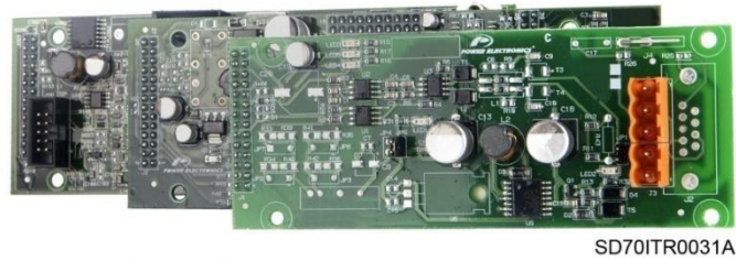
Figure 12.1 Example of Profibus optional board
