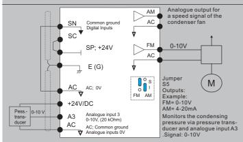
**Speed controll of a condensing unit;** R134A; 10,0 Bar pressure. Sensor 2: Transducer 0,0 Bar to 18 Bar connected at A3 (Condenser pressure) P6-01 = 0,0 Bar (Lower value pressure transducer, Cond. pressure) P6-02 = 18,0 Bar (Eugen value pressure transducer, Cond. pressure) P6-03 = 10,0 Bar (Reference pressure condenser) P6-05 = 5,0 (P-gain PI control) P6-06 = 10s (I-time PI control)
