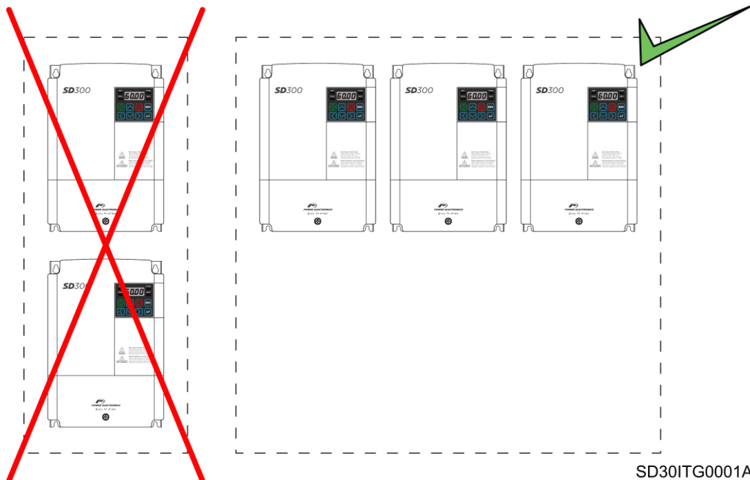
Figure 6.3 Installing multiple drives
